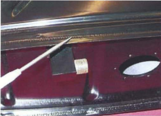
Continuous [resistance] weld at tank ends. High quality look to welds
