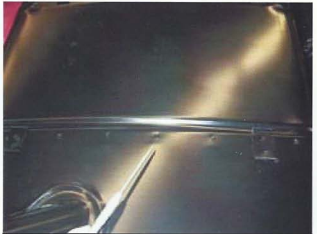
Internal baffles spot welded as original tanks; on previous tanks the internal baffles were MIG welded
