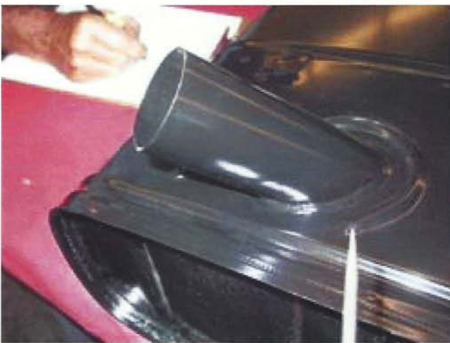
High quality weld at filler neck.
